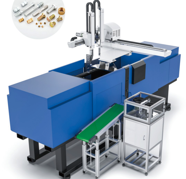
各类螺母埋入注塑 All kinds of nuts are embedded in injection molding
